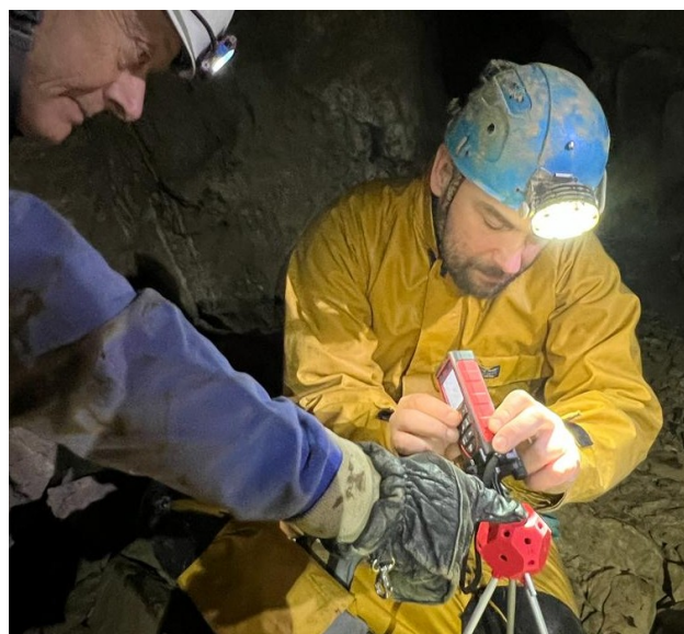
Figure 28: Calibration of a Disto-X2 using a 3D-printed calibration cube. Photo by Erik Claes.
