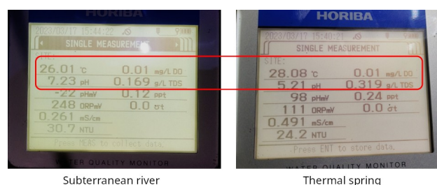
Figure 19: Comparison of water measurements between subterranean river and spring. Photo by Dan Husana.
